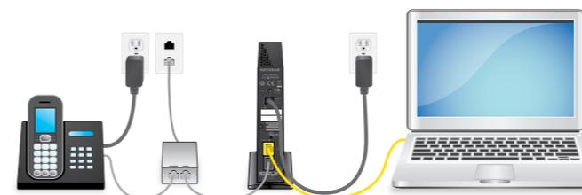
Use the Ethernet cable to connect a computer to the yellow LAN port on your DSL modem.
