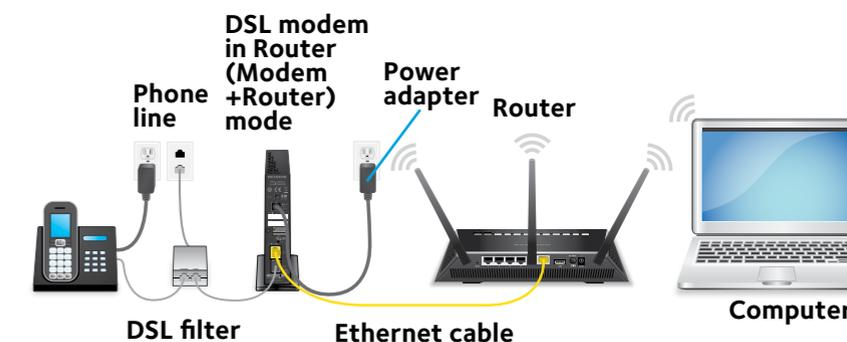
Disconnect the computer from your DSL modem and use the Ethernet cable to connect the yellow LAN port on your DSL modem to the WAN port on a router.
