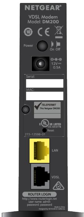
2. Using a straightened paper clip, press and hold the **Reset** button for at least five seconds.
